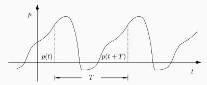
Fourier theorem asserts that periodic loadings can be represented by an infinite series of harmonic functions. E.g., for an antisymmetric periodic loading of period T we have a series composed of antisymmetric harmonic functions
