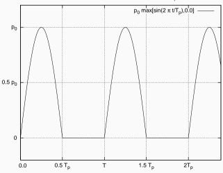
As an example, consider the loading  $p(t) = \max\{p_0 \, \sin \frac{2\pi t}{T_{\rm D}}, \, 0\}$
