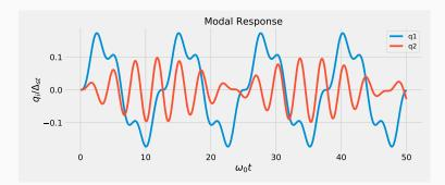
In the graph above, the responses are plotted against an adimensional time coordinate  $\alpha$  with  $\alpha=\omega_0 t$ , while the ordinates are adimensionalised with respect to  $\Delta_{\rm st}=\frac{p_0}{k}$
