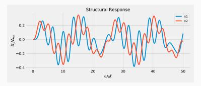
And the displacement of the centre of mass plotted along with the difference in displacements.
