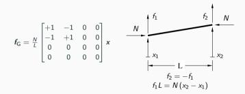
Using *FEM*, with the previous shape functions, by PVD it is  $k_{G,ij} = \int N(s)\phi'_i(s)\phi'_j(s) ds$ , leading, for constant N, to
