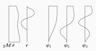
For EQ loading,  $\Gamma_1$  is relatively large for the first mode, as loading components and displacements have the same sign, with respect to other  $\Gamma_i$ 's, where the oscillating nature of the higher eigenvectors will lead to increasing cancellation.
