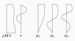
Consider a shear type building, its first 3 eigenvectors as sketched above, with mass distribution approximately constant over its height and its earthquake load shape vector
