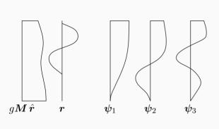
For EQ loading,  $\Gamma_1$  is relatively large for the first mode, as loading components and displacements have the same sign, with respect to other  $\Gamma_i$ 's, where the oscillating nature of the higher eigenvectors will lead to increasing cancellation.
