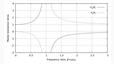
For a fixed excitation frequency and high modal frequencies the frequency ratio  $\beta \to 0.$
