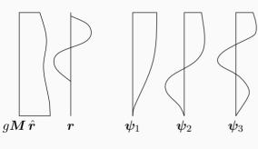
Consider a shear type building, its first 3 eigenvectors as sketched above, with mass distribution approximately constant over its height and its earthquake load shape vector
