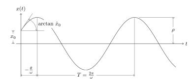
It is worth noting that the coefficients A, B and C have the dimension of a length, the coefficient  $\omega_n$  has the dimension of the reciprocal of time and that the coefficient  $\varphi$  is an angle, or in other terms is adimensional.
