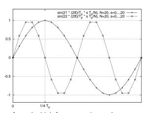
See the plot above: the contributions from the high frequency sines, when sampled, are indistinguishable from the contributions from lower frequency components, i.e., are aliased to lower frequencies!
