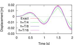
It is apparent that you have a very good approximation when the linearised loading is a very good approximation of the input function oscillator
