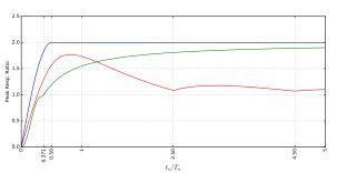
rectangular triangular half sine SDOF linear oscillator
