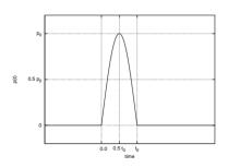
where  $\omega = \frac{2\pi}{2t_0}$  is the frequency associated with the load.
