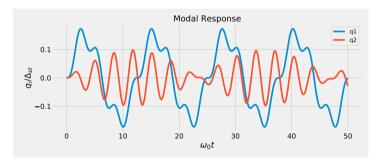
In the graph above, the responses are plotted against an adimensional time coordinate  $\alpha$  with  $\alpha=\omega_0 t$ , while the ordinates are adimensionalised with respect to  $\Delta_{\rm st}=\frac{p_0}{k}$
