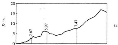
The response spectrum is a plot of the peak values of a response quantity, say the displacement response function, computed for different values of  $T_n$  and the same  $\zeta$ , versus natural period  $T_N$ .
