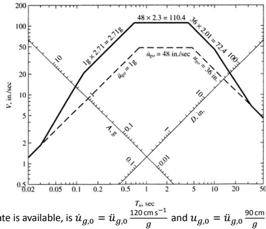
A common assumption, used when only the  $\ddot{u}_{g,0}$  estimate is available, is  $\dot{u}_{g,0} = \ddot{u}_{g,0} \frac{120 \text{ cm s}^{-1}}{g}$  and  $u_{g,0} = \ddot{u}_{g,0} \frac{90 \text{ cm}}{g}$ .
