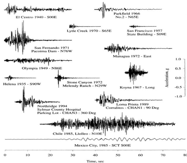
A number of different strong motion records, recorded at different sites and due to different earthquakes, are plotted with the same scale, both in time and in acceleration.
