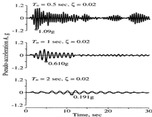
Left, pseudo accelerations computed for varying  $T_n$ . Compare with previous page's figure. The relative magnitudes are reverted: for  $T_n = 0.5$  s we have a maximum force and a minimum displacement, while for  $T_n = 2.0$  s the force is minimum and the displacement maximum.
