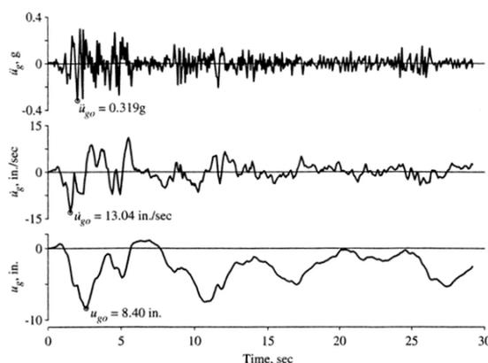
**Figure 6.1.4** North-south component of horizontal ground acceleration recorded at the Imperial Valley Irrigation District substation, El Centro, California, during the Imperial Valley earthquake of May 18, 1940. The ground velocity and ground displacement were computed by integrating the ground acceleration.
