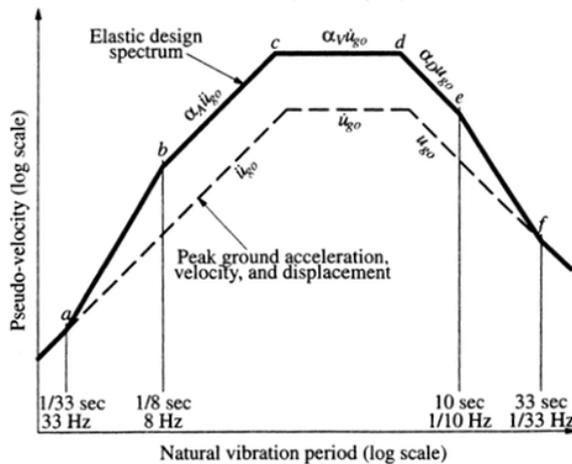
The key periods  $T_a = 0.03 \text{ s}$  and  $T_b = 0.125 \text{ s}$  define the segment where  $A$  rises from 1 to  $\alpha_A$ .
