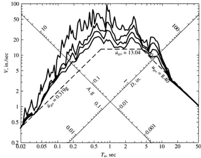
The El Centro 1940 NS  $D - V - A$  spectrum, *plus* three lines corresponding to the peak values of the ground acceleration, ground velocity and ground displacement.
