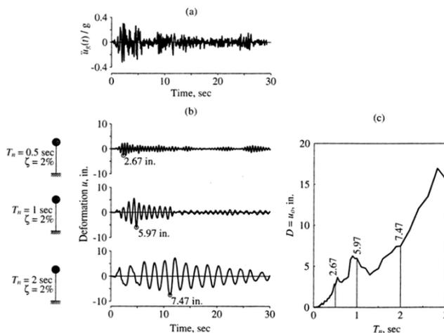
For a fixed values of  $\zeta$  (usually one of 0% 0.5% 1% 2% 3% 5% 7% 10% 15% and 20%) and for variable values of  $T_n$  (usually ranging from 0.01 s to 20 s)
