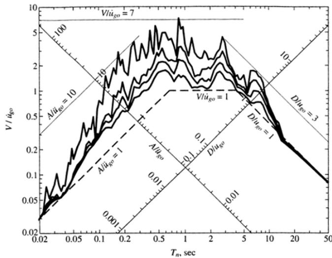
First step in the construction of an idealized  $D - V - A$  response spectrum is to make a tripartite plot with all three ordinate axes normalized with respect to  $u_{g,0}$ ,  $\dot{u}_{g,0}$  and  $\ddot{u}_{g,0}$ .
