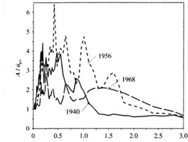
For design purposes, however, it is not necessary to know in advance and in detail the next quake's response spectra as it suffices to know some sort of an upper bound on spectral ordinates, that is a *Design Spectrum*.
